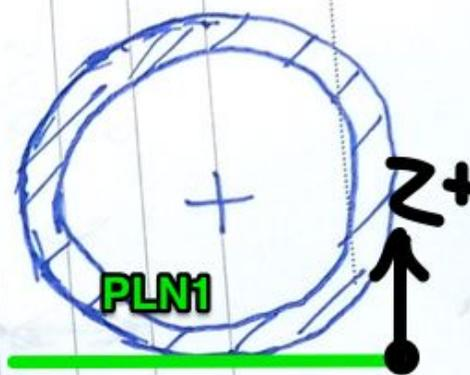
2) create auto circle (1, 2) with reference feature PLN1, construct line (LIN1), set LIN1 as Y+, translate X+ to LIN1, translate Y+ to CIR1, create alignment; check if probe moving in wrong direction (Z- instead of Z+ or X- instead of X+), then change vector K direction (+ to -) in PLN1 settings (F9)
