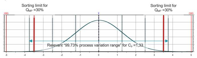
What makes things even worse is that 100% inspections only require a capability index of  $C_p = 1$ . The produced number of rejects amounting to 2700 ppm thus increases to an "inspected" number of rejects of 35730 ppm.
