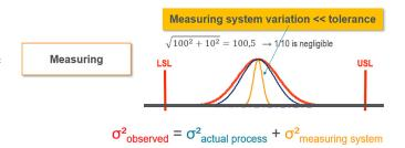
A different application is the conformity assessment of single parts. We pick one measured value of each part, compare this very value to the specification and make a test decision. We thus use the measurement process to gain a piece of information about a part and compare this information later on to the specified limits for analysis purposes.
