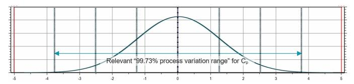
If we permit the capability ratio to amount to  $Q_{MP} \le 30\%$  and stick to the 100% inspection, we may only release parts within a 70% zone of the tolerance. In case the declared excess proportion is now also supposed to be less than 63 ppm, 99.9957% of all values ("8s") need to be within the 70% zone, e.g. your processes must have a capability index of  $C_p = 1.9$ . Does this make sense? Rather not.
