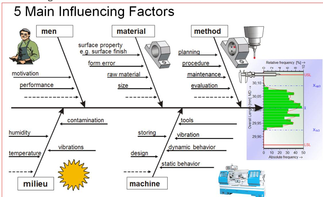
The phase of process qualification is typically a two-stage process. The first stage helps to find the ideal performance of the machine (or manufacturing equipment – it does not have to be a “machine“, it can also be a filling device or a technical process). This phase does not consider any influences other than the actual machine, i.e. it eliminates other influences or keeps them constant.
