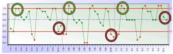
This diagram makes it clear that the tenth part shows a huge difference that is more considerable compared to all the other parts (as an example, we also highlighted the second part). The diagram below displaying the deviations of each individual measurement from the mean of the respective part shows it even more clearly.
