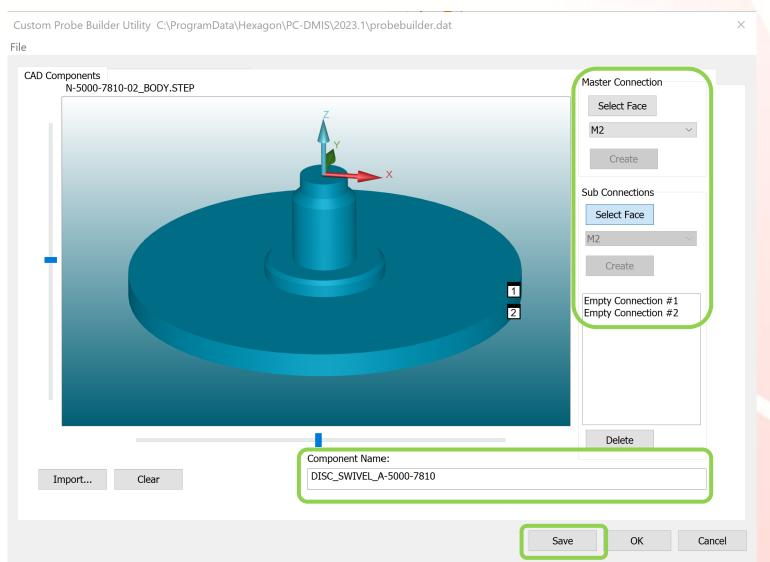
Once the model is imported, you then must establish the type and location of connections.
