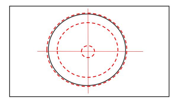
Explanation why the MMP value here is 0 at the natural boundaries: even more joining capacity is not possible. Any larger and the diameter of the hole would be outside the specification limit.
