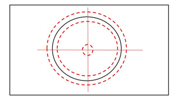
Explanation why the value of the MMP group is not 0 here: for maximum joining ability, the diameter of the hole could still be 0.2 larger.
