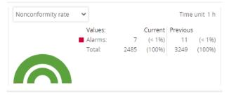
The nonconformity rate shows the number of measured values with alarm as a percentage of all measured values from the Current time unit.
