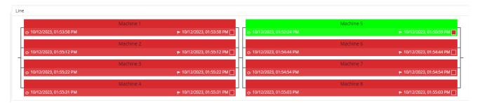
Each machine shows the status of the last measurement (green/yellow/red). The right part of each machine tile shows when the last alarm occurred.
