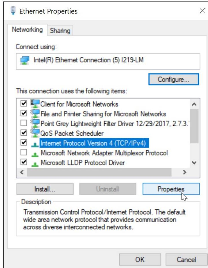
4. Inside the properties, use the following IP Address to 128.128.128.10 (10-99) and the subnet mask to 255.255.255.0 as shown below and press **OK** to accept the configuration. If you changed the IP address of your FARO tracker, please enter in the value here from the utilities.
